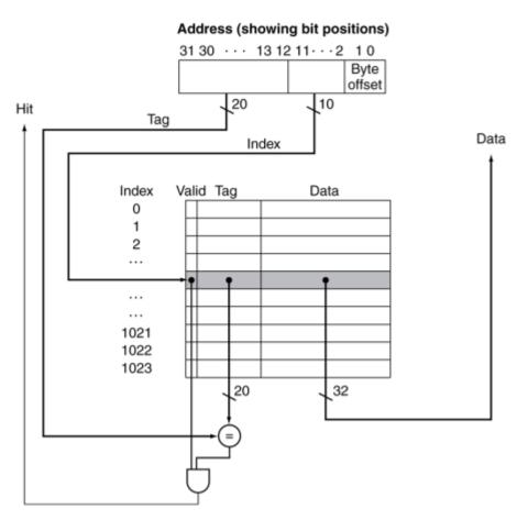
The comparator Circuit through which tag is compared with specified bits of address:
